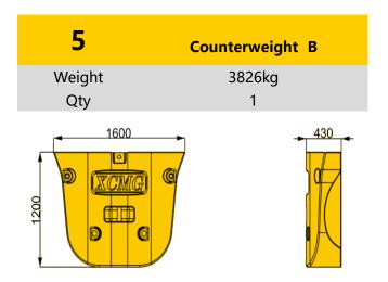
NOTES: All of these are single piece weight, and boom assembly include boom and telescopic cylinder.
